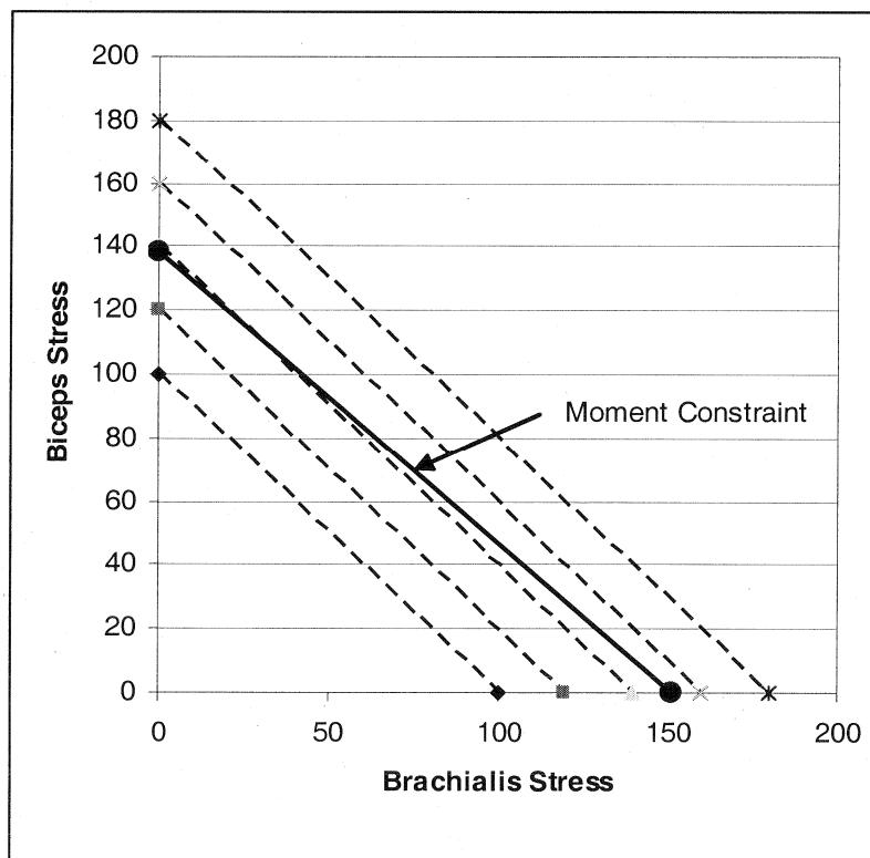
Plotting values of the objective function  $S_{TOT} = S_{BR} + S_{BI} = \text{constant}$ , along with the moment equation demonstrates that the minimum stress will occur at the point where the Brachialis stress is zero and the Biceps stress is  $138.5 \text{ N/cm}^2$ , corresponding to a force of 622.6 N.
